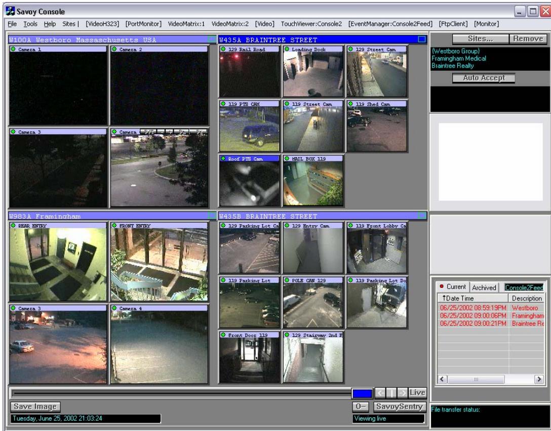
Figure 1 Savoy's Console showing video from four servers across three remote sites
